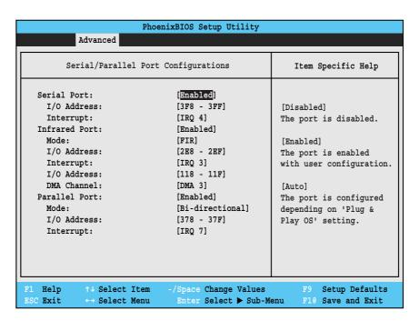
Figure 4. Serial/Parallel Port Configurations Submenu
